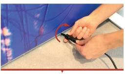
**11.** Link the power supply cable to the plug at the backside of the frame and twist the cap to secure the connection.
