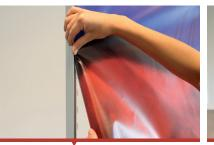
Attach the fabric on both sides, by pushing the silicone edges in the grooves.
