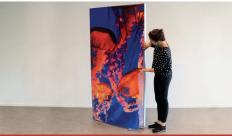
10. Start in the corners to divide the tension and work your way around the frame until all silicone edges are attached.
